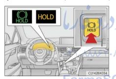
Turns the brake hold system on
