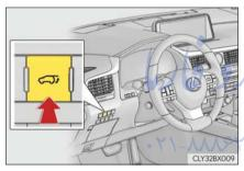
To open or close the power back door, press and hold the switch for approximately 1 second.
