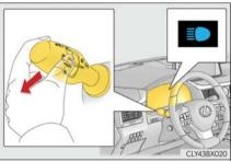
1 Push the lever away from you with the headlight switch in the O or AUTO position.
