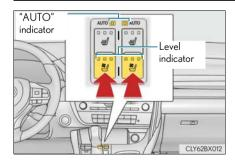
When any switch is pressed, the system is set to automatic mode and the "AUTO" indicator (green) lights up.
