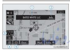
To scroll over the map, place the cursor mark in the desired position and then press and hold the Remote Touch knob.
