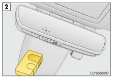
Point the remote control transmitter for the device at the rear view mirror, 1 to 3 in. (25 to 75 mm) from the HomeLink  $^{\circledR}$  buttons. Keep the HomeLink  $^{\circledR}$  indicator light in view
