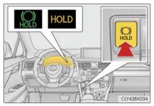
Turns the brake hold system on
