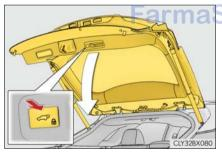
To close the power back door, press the switch.
