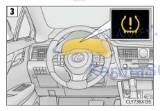
Press  $\wedge$  or  $\vee$  of the meter control switch, select the "TPMS" screen and then press and hold the until the tire pressure warning light blinks slowly 3 times.
