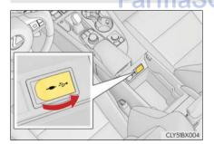
Press the console box knob, open the cover and connect the portable audio device.
