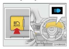
Press the Automatic High Beam switch.
