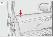
With the door open, push down the inside lock button.
