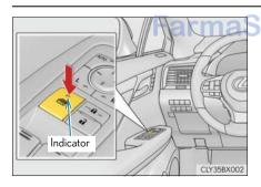
Press the switch down to lock the passenger windows. The indicator light will come on when the passenger windows are locked.
