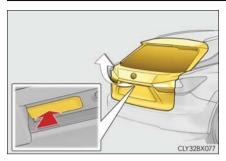
When the power back door is unlocked: Press the back door opener switch.
