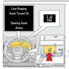
Press the LKA switch to turn the LKA system on.
