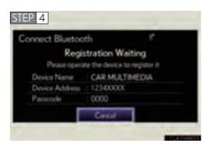
When this screen is displayed, input the passcode displayed on the screen into your Bluetooth® device.
