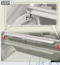
Push from above until the claws on both sides are securely locked in position.
