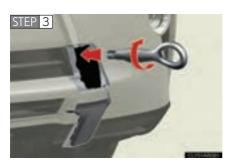
Insert the towing eyelet into the hole and tighten as much as possible by hand.
