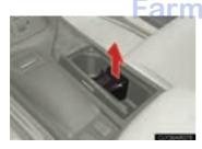
The cup holder insert may be removed for cleaning.
