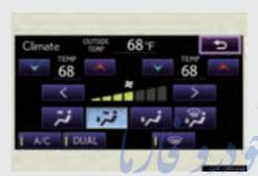
The outside temperature is displayed on the air conditioning operation screen.  $(\rightarrow P. 345)$
