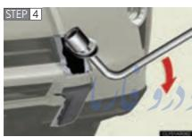
Using the tip of the wheel nut wrench, tighten down the towing eyelet securely without interfering with the bumper.
