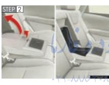
Pull up the lever to release the lock and lift the armrest.
