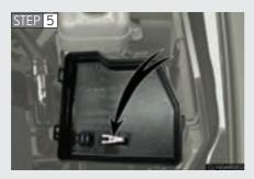
Remove the fuse with the pullout tool.
