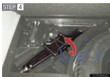
Remove the jack after removing the hook.
