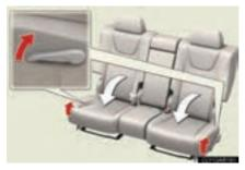
Pull the seatback angle adjustment lever.
