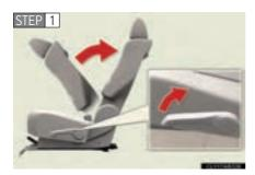
Fold the seatback while pulling the seatback angle adjustment lever. Return the seatback and secure it at the first lock position. (→P. 72)
