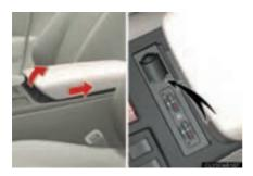
Pull up the lever to release the lock, and slide the armrest.
