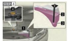
The coolant level is satisfactory if it is between the "FULL" and "LOW" lines on the reservoir.
