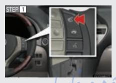
Press and hold the off hook switch until you hear the beeps that indicate the system is listening.
