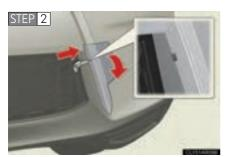
Insert the mechanical key ( $\rightarrow$ P. 31) into the groove and release the claws. With the mechanical key inserted, remove the eyelet cover by pulling it towards you.
