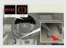
To set the parking brake, fully depress the parking brake pedal with vour left foot while depressing the brake pedal with your right foot.
