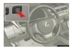
Switches between odometer and trip meter displays. When the trip meter is displayed, pressing and holding the button will reset the trip meter.
