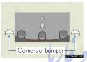
The area detected by the camera is limited. Object which are close to either corner of the bumper or under the bumper cannot be seen on the screen.
