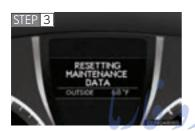
Keep the "ODO/TRIP" button pressed for about 5 seconds. The resetting procedure is complete when "OOOOO0" in the trip meter flashes once and the message in the multi-information display disappears.
