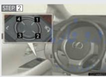
To adjust the mirror, press the switch.
