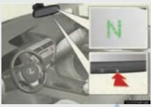
To turn the compass on or off, press for more than 3 seconds.
