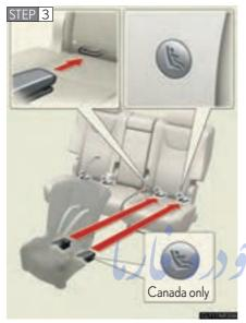
Latch the buckles onto the LATCH anchors. If the child restraint has a top tether strap, the top tether strap should be latched onto the top tether strap anchor bracket.
