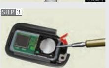
Remove the depleted battery.
