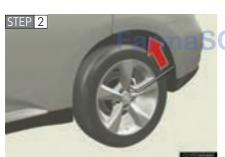
Slightly loosen the wheel nuts (one turn).
