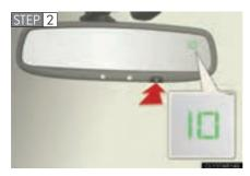
The location the compass is displayed differs according to the type of inner rear view mirror.
