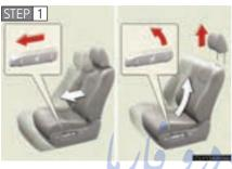
Move the front seat forward, raise the seat, and remove the head restraint.  $(\rightarrow P. 81)$
