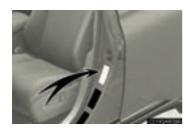
For the GAWR, see the Certification Label. For the maximum load of the tire, see the load limit at maximum cold tire inflation pressure mentioned on the sidewall of the tire. (→P. 821)
