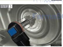
Replace the light bulb, and install the bulb base.
