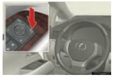
Press the switch to fold the mirrors.
