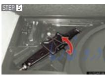
Remove the jack after removing the hook.
