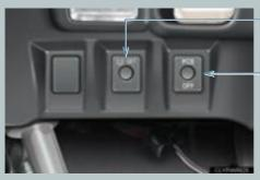
Tire pressure warning reset switch P.686
