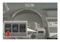
Pressing the switch turns the headup display on/off and changes the vehicle speed display units as follows:
