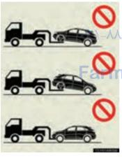
Be sure to transport the vehicle with the front wheels raised or with all four wheels raised off the ground.
