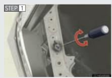
Turn bolt A in either direction using a Phillips-head screwdriver.
