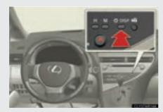
Press and release the "DISP" switch until the brightness of the display is adjusted to the desired level.
