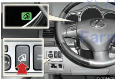
To turn the easy access mode on and off, press the easy access mode switch.
