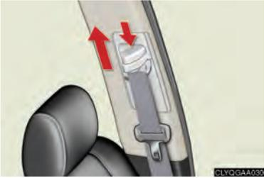
To raise: push the anchor upward.
