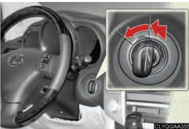
The steering wheel locks when the engine switch is turned to the LOCK position.
