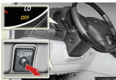
To cancel the height control, press the height control switch. The indicator light comes on and the vehicle height is fixed.
