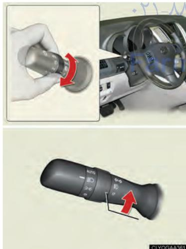
The fog lights can be used only when the headlights (low beam) are on.
