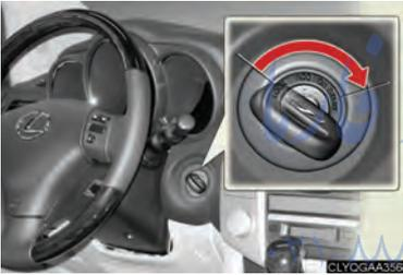
2 Turn the engine switch to the START position.
