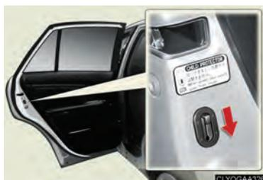
Setting the switch to the LOCK position prevents the rear doors from being opened from the inside.
