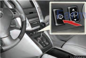
The headlight cleaner can be used only when the engine switch is in the ON position and the headlights are on.
