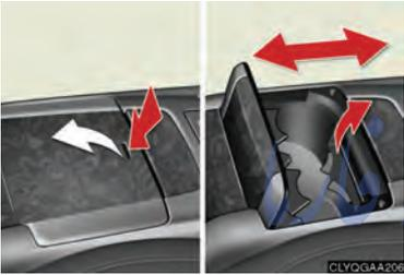
To adjust the position of the front console box, open the cup holder lid and slide the console box while lifting the lever.
