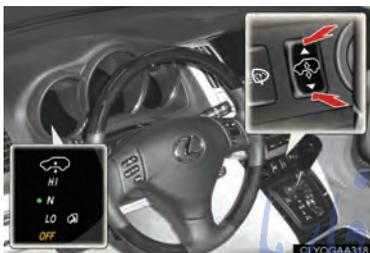
To select a height mode, press ▲ or ▼ on the height select switch.
