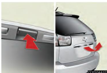
To open the back door, push up the opener and raise the door.
