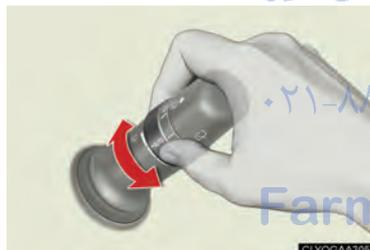
Automatic operation: Sensitivity can be adjusted by turning the band.
