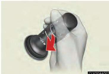
To spray washer fluid, pull the lever. The wipers will operate automatically.
