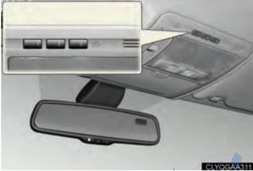
The HomeLink® compatible transceiver in your vehicle has 3 buttons which can be programmed to operate 3 different devices.
