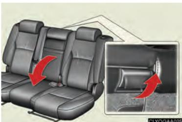
Pull the lever behind the center seatback and fold the seatback down.
