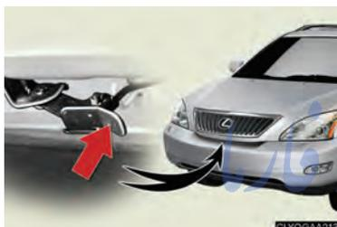
2 Insert your fingers under the hood, pull the hood catch and lift the hood.
