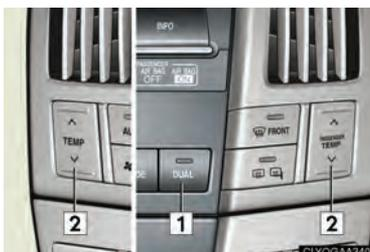
In DUAL mode, driver and passenger side temperature settings can be adjusted separately.
