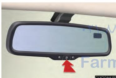
To turn the anti-glare function ON/OFF, press and hold the button for 3 seconds.
