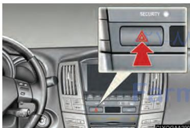
Engaging the emergency flasher switch causes all the turn signal lights to flash. The emergency flashers can be operated even when the engine is off.
