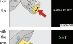
Accelerate or decelerate, with accelerator pedal operation, to the desired vehicle speed (above approximately 50 km/h [30 mph]) and push the lever down to set the speed.
