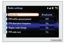
When alternative frequency is set to on, a station providing good reception is automatically selected if current reception worsens.
