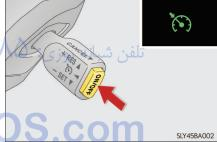
Accelerate or decelerate, with accelerator pedal operation, to the desired vehicle speed (above approximately 40 km/h [25 mph]) and push the lever down to set the speed.
