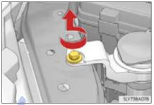
When it is difficult to work, remove the washer fluid supply opening.
