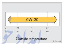
Oil viscosity (OW-20 is explained here as an example):
