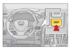
On and off will be switched between each time the button is pressed. If the button is left alone without being operated for a short time, setting will be finished automatically.
