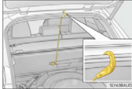
When attaching the side deck board, attach it so that the "↑FRONT" mark points to the front side of the vehicle.
