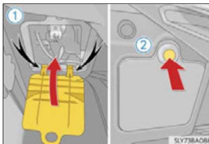
**9** Install the engine compartment cover. (→P. 491)
