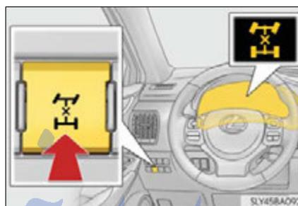
■ **All-wheel drive lock mode can be operated when**
