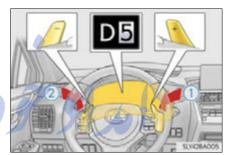
To return to normal  $\mathsf{D}$  position driving, the "+" paddle shift switch must be held down for a period of time.
