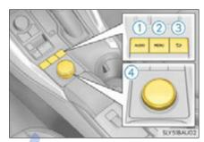
Move the controller to display the left or right side of the screen. Push the controller to enter the selected function and number.
