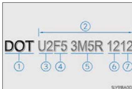
\*: The DOT symbol certifies that the tire conforms to applicable Federal Motor Vehicle Safety Standards.
