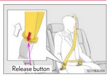
Insert the mechanical key (→P. 108) or plate B into the notch of buckle A and remove the belt.
