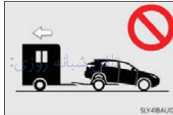
AWD models: Never tow this vehicle with any of the wheels on the ground. This may cause serious damage to the transmission and Dynamic Torque Control AWD system.
