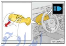
2 Press the Automatic High Beam switch.
