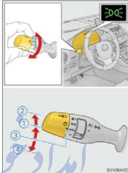
**Turning on the high beam headlights**
