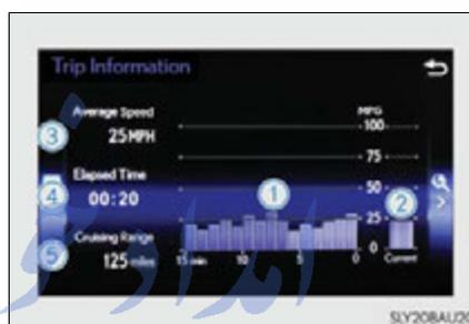
Average fuel consumption for the past 15 minutes is divided by color into past averages and averages attained since the engine switch was last turned to IGNITION ON mode. Use the displayed average fuel consumption as a reference.
