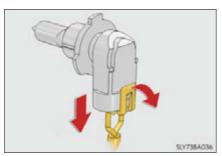
5 Confirm whether the O-ring of the cover has not come off. If the O-ring come off, attached to the proper position.
