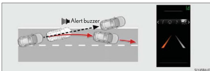
When the system judges that the vehicle is deviating from the current traffic lane, an alert buzzer sounds and it prompts cautions from the display screen of the multi-information display.
