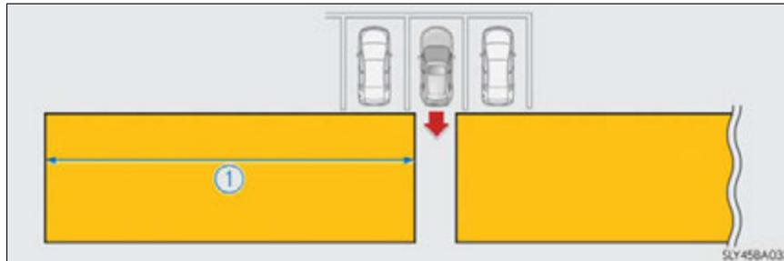
To give the driver a more consistent time to react, the buzzer can alert for faster vehicles from farther away.
