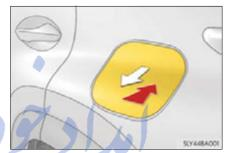
2 Turn the fuel tank cap slowly to open and put it into the holder on the fuel filler door.
