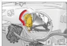
4 Unplug the connector while pulling the lock release.
