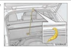
When attaching the side deck board, attach it so that the "TRONT" mark points to the front side of the vehicle.
