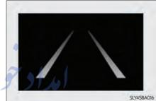
When the either lane line turns white: Indicates that the lane marker on the white-marked side is recognized.
