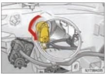
4 Unplug the connector while pulling the lock release.
