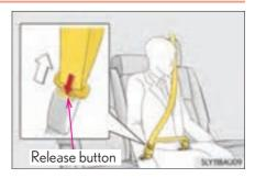
Insert the mechanical key  $(\rightarrow P. 108)$  or plate B into the notch of buckle A and remove the belt.
