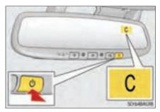
a) Drive the vehicle at 5 mph (8 km/h) or less in a circle until a direction is displayed.
