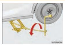
**5** Firmly tighten each wheel nut two or three times in the order shown in the illustration.
