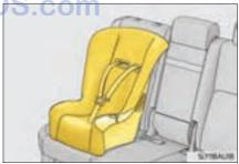
4 Run the seat belt through the child restraint system and insert the plate into the buckle. Make sure that the belt is not twisted.
