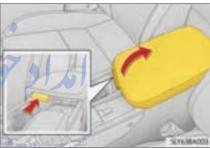
Vehicles with the wireless charger: Lift the wireless charger.
