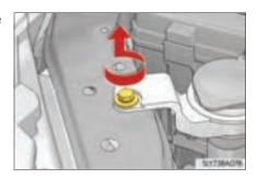
When it is difficult to work, remove the washer fluid supply opening.
