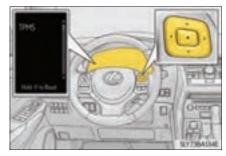
A message and an indicator are displayed by the multi-information display, and initialization is completed.
