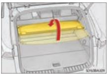
3 Pull the lever upwards and open the deck board.
