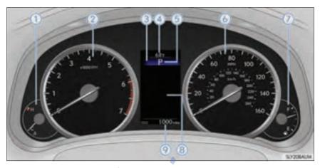
1) Engine coolant temperature gauge
