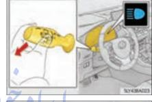
**2** Press the Automatic High Beam switch.
