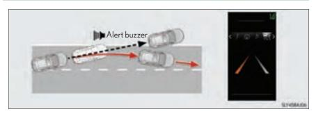
When the system judges that the vehicle is deviating from the current traffic lane, an alert buzzer sounds and it prompts cautions from the display screen of the multi-information display.
