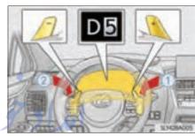
To return to normal D position driving, the "+" paddle shift switch must be held down for a period of time.
