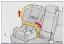
7 After installing the child restraint system, rock it back and forth to ensure that it is installed securely.
