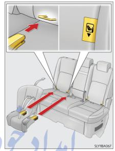
After installing the child restraint system, rock it back and forth to ensure that it is installed securely.
