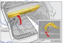
Attach the hook to the upper edge of the back door opening as shown.
