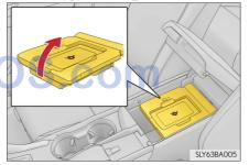
• Vehicles without the wireless charger: The tray slides forward/backward and can be removed.
