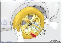
Vehicles with a full-size spare tire: Remove the wheel ornament by pushing from the reverse side.
