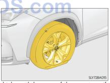
• To avoid sealant leakage, move the vehicle until the area of the puncture, if known, is positioned at the top of the tire.
