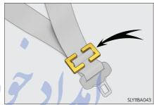
After installing the child restraint system, rock it back and forth to ensure that it is installed securely.
