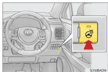
Turns the heated steering wheel on/off
