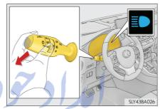
**2** Press the Automatic High Beam switch.
