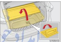
4 Lift the deck board and remove the hook on the backside of the deck board.
