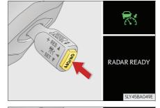
Accelerate or decelerate, with accelerator pedal operation, to the desired vehicle speed (above approximately 50 km/h [30 mph]) and push the lever down to set the speed.
