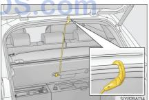
**6** Take out the emergency tire puncture repair kit.
