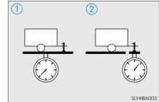
Allocate the trailer load so that the drawbar load is greater than 25 kg (55.1 lb.) or 4% of the towing capacity. Do not let the drawbar load exceed the indicated weight. ( $\rightarrow$ P. 628)
