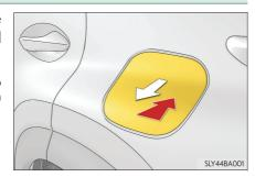
Turn the fuel tank cap slowly to remove it and put it into the holder on the fuel filler door.
