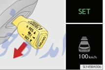
While the vehicle is in vehicle-to-vehicle distance control mode, if the lever is released when vehicle speed is less than 50 km/h (30 mph) and a vehicle ahead can be detected, the vehicle will start following the vehicle ahead at a set speed of 50 km/h (30 mph).
