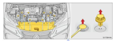
■ Installing the clips
