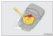
4 Remove the depleted battery. Insert a new battery with the "+" terminal facing up.
