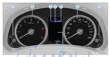
1 Engine coolant temperature gauge
