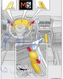
However, even when in the M position, the gear steps will be automatically changed if the engine speed is too high, or too low.
