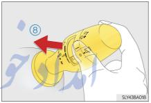
■ The windshield wipers and washer can be operated when The engine switch is in IGNITION ON mode.
