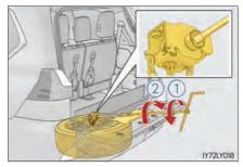
4 Lower the spare tire completely to the ground.
