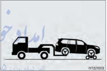
Use a towing dolly under the rear Use a towing dolly under the front wheels.
