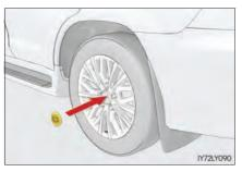
Remove the center wheel ornament from the flat tire by pushing from the reverse side, and reinstall it.
