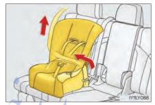
6 If the child restraint system has a top tether strap, the top tether strap should be latched onto the top tether strap anchor.  $(\rightarrow P. 71)$
