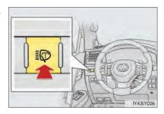
■ The headlight cleaners can be operated when The engine switch is in IGNITION ON mode and the headlight switch is turned on.
