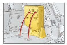
If the switch is held down the seat will automatically return to the folding position. (Buzzer sounds twice)
