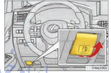
2 Turn the fuel tank cap slowly and remove it, then put it into the holder on the fuel filler door.
