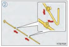
3 Assemble the jack handle extension bar and the jack handle and tighten the screw.
