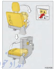
Remove the seat hook covers from the underside of the seat cushion, and install them on the
