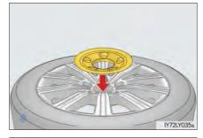
2 Install the holding bracket, inserting the claw into the wheel lug nut hole. Turn the jack handle extension clockwise to take up slack in the chain.
