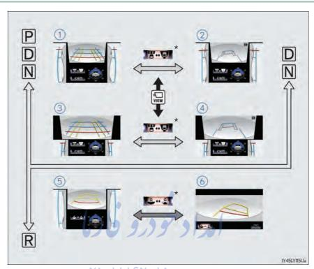
1) Front view & dual side view: Under vehicle terrain view & dual →P. 327 side view (front magnified):
