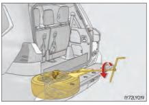
**5** Pull out the spare tire and remove the holding bracket and spare wheel cover.
