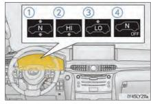
When the height control "OFF" indicator is displayed, the vehicle height will not change even if the height select switch is operated.
