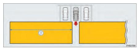
The buzzer can alert the driver of faster vehicles approaching from farther away. Example:
