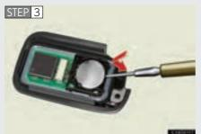
Remove the depleted battery.
