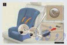
1 Child LATCH restraint anchors
