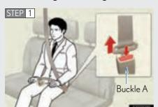
Push the release button on buckle A
