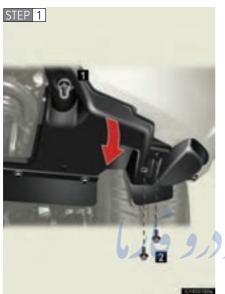
Remove the fender liner bolts, loose the fender liner nut and remove the fender liner.
