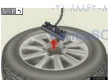
Pull out the spare tire and remove the holding bracket.
