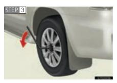
Slightly loosen the wheel nuts (one turn).
