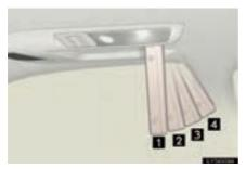
The display angles change as follows each time "TILT" is pressed.
