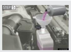
Add engine coolant if necessary.
