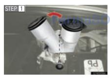
For the left side only: Remove the securing bolt and move the washer fluid filler opener.
