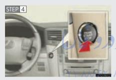
Press the "ENGINE START STOP" switch.
