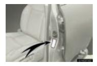
For the GAWR, see the Certification Label. For the maximum load of the tire, see the load limit at maximum cold tire inflation pressure mentioned on the sidewall of the tire.  $(\rightarrow P.711)$
