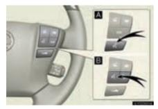
Press to operate the voice command system. (→"Navigation System Owner's Manual")
