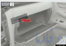
Open the glove box and remove the filter cover.
