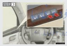
While pressing the "SET" button, or within 3 seconds after the "SET" button is pressed, press and hold button "1", "2" or "3" until the signal beeps.
