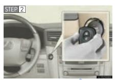
Touch the Lexus emblem side of the electronic key (including the card key) to the "ENGINE START STOP" switch.
