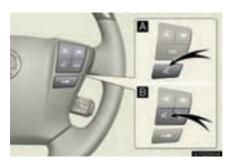
Press or to operate the voice command system. (→"Navigation System Owner's Manual")
