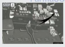
Remove the fuse with the pullout tool.
