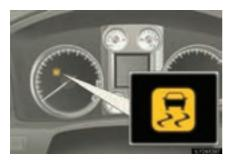
If the vehicle is in danger of slipping, rolling backwards when starting on an incline, or if the wheels spin, the slip indicator light flashes to indicate that the VSC/Active TRAC/hill-start assist control systems have been engaged.
