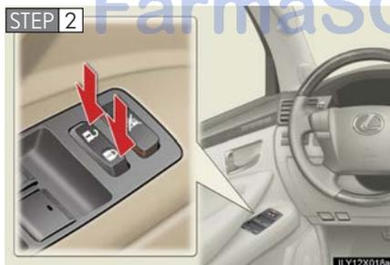
Shift the shift lever to "P" or "N", and press and hold the driver's door lock switch (
