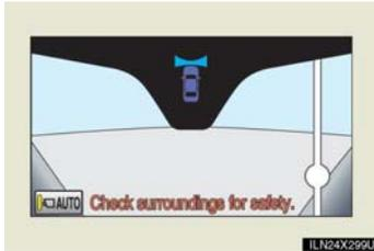
If a bright light (for example, sunlight reflected off the vehicle body) is picked up by the camera, a smear effect\* peculiar to the camera may occur.
