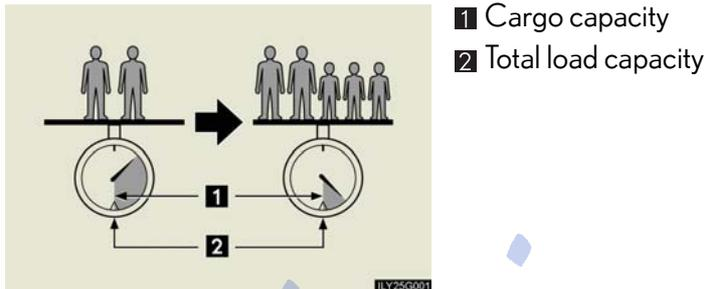
When 2 people with the combined weight of 366 lb. (166 kg) are riding in your vehicle, which has a total load capacity of 1230 lb. (560 kg), the available amount of cargo and luggage load capacity will be as follows:
