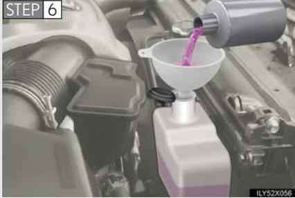
Add engine coolant if necessary.
