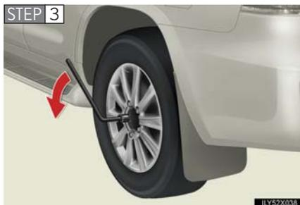
Slightly loosen the wheel nuts (one turn).
