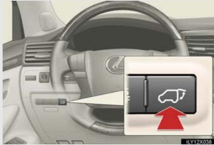
The power back door can be opened/closed using the power back door switch or wireless remote control. (→P. 45)
