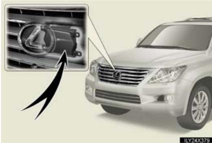
When traveling on a road with very light traffic and very little to reflect the radar waves emitted by the radar sensor, the system may decide that the radar sensor is dirty, even if the sensor is not actually dirty. The system will automatically restore itself when reflected radar waves are detected.
