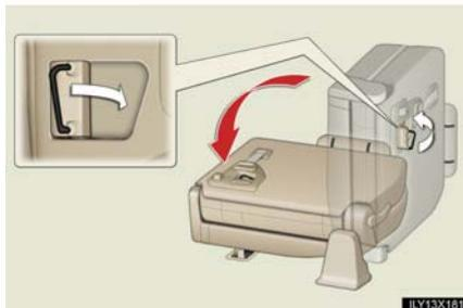
The seatback striker will be automatically stowed when the seat is lowered.
