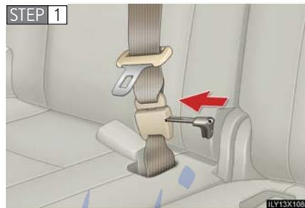
To release the hooked tab, insert the mechanical key into the hole on the buckle with the light gray buckle release button.
