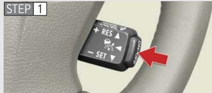
Press the "ON-OFF" button to activate the cruise control.
