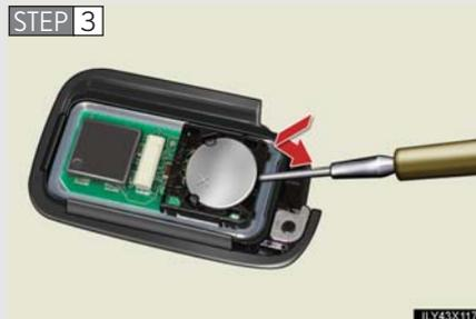
Remove the depleted battery.
