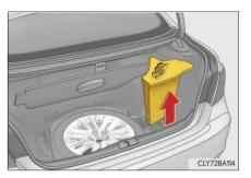
Remove the jack after removing the hook.
