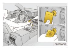
Press the engine switch within 10 seconds of the buzzer sounding, keeping the brake pedal depressed.
