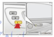
Seat return operation after turning the engine switch off The seat will automatically return to the neutral position if the door is opened within approximately 45 seconds of the engine switch being turned off.
