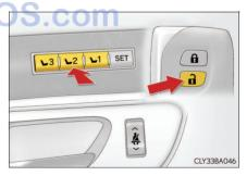
To prevent unintended triggering of the alarm, open and close a door once after a driving position has been recorded. (If a door is not opened within 30 seconds after is pressed, the doors will be locked again and the alarm will automatically be set.)
