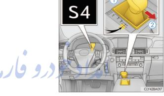
The initial shift range in S mode is set automatically between 3 and 7 according to vehicle speed and driving conditions.
