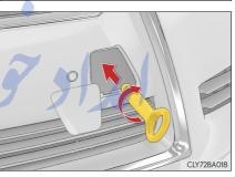
4 Tighten down the towing eyelet securely using a wheel nut wrench or hard metal bar.
