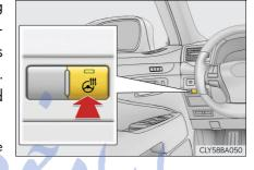
The indicator light comes on when the heater is operating.
