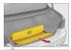
Take out the emergency tire puncture repair kit.
