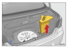
3 Remove the jack after removing the hook.
