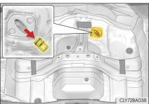
**7** Replace the screwdriver head with the parking brake release tool.
