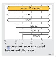
Oil viscosity (OW-20 is explained here as an example):
