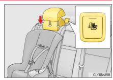
2 Open the anchor bracket cover, latch the hook onto the anchor bracket and tighten the top strap.
