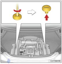
4 While lifting the inner corners of the right and left side deck boards, pull out the tool tray.
