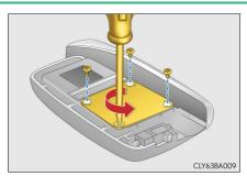
Remove the depleted battery.
