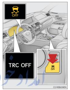
\*: On vehicles with pre-crash safety system, pre-crash alert braking, pre-crash brake assist and pre-crash braking will also be disabled. The pre-crash safety system warning light will come on and the "Pre-crash brakes are disabled because VSC is OFF" will be shown on the multi-information display. (
