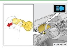
**2** Press the Adaptive High-beam System switch.
