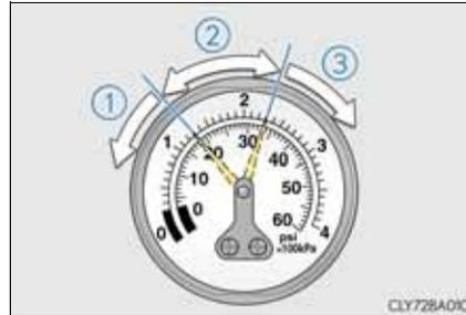
① If the tire inflation pressure is below 130 kPa (1.3 kgf/cm<sup>2</sup> or bar, 19 psi): The puncture cannot be repaired. Contact any authorized Lexus dealer or repairer, or another duly qualified and equipped professional.
