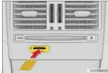
To eject the SD card, push on the center of the SD card. When it is ejected slightly, pull it straight out.
