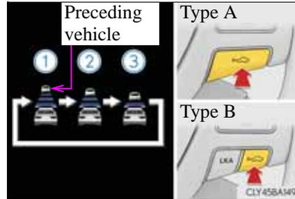
The vehicle-to-vehicle distance is set automatically to long mode when the engine switch is turned to IGNITION ON mode.
