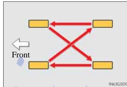
To equalize tire wear and help extend tire life, Lexus recommends that tire rotation is carried out approximately every 10000 km (6000 miles) for 2WD models or 5000 km (3000 miles) for AWD models.
