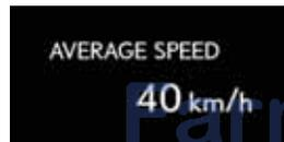
Displays the average vehicle speed since the function was reset
