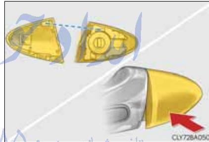
Make sure that the lower claw of the cover is securely fastened to the lower catch on the vehicle side. If the cover is not securely attached, it may fall off while driving.
