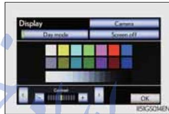
If the screen is set to day mode with the headlight switch turned on, this condition is memorized even with the engine turned off.
