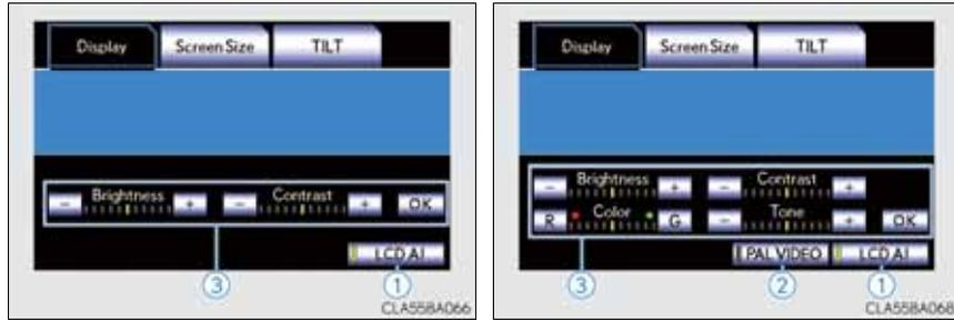
① Turning on/off the “LCD AI”
