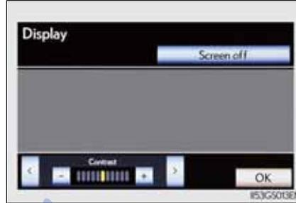
The screen goes off when “Screen off” is selected. To turn the display screen back on, press any button on the audio panel or on the Remote Touch. The selected screen appears.
