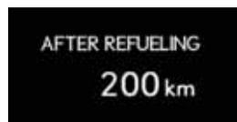
Displays the distance the vehicle has been driven since the vehicle was last refueled
