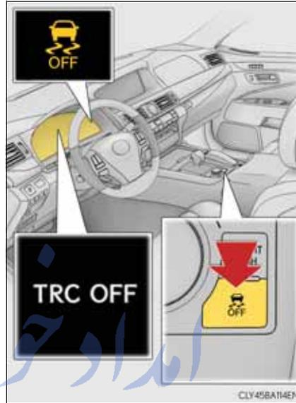
\*: On vehicles with pre-crash safety system, pre-crash alert braking, pre-crash brake assist and pre-crash braking will also be disabled. The pre-crash safety system warning light will come on and the “Pre-crash brakes are disabled because VSC is OFF” will be shown on the multi-information display. (→P. 355)
