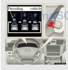
Pressing the button changes the vehicle-to-vehicle distance as follows:
