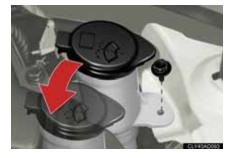
Remove the securing bolt and move the washer fluid filler opening.
