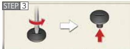
Using the flathead end of the screwdriver, remove the clips.
