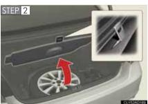
Secure the panel using the hook provided.
