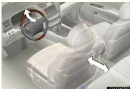
The auto away/return function enables easy access by activating when the driver attempts to enter or exit the vehicle.
