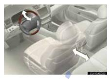
The auto away/return function enables easy access by activating when the driver attempts to enter or exit the vehicle.
