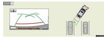
Back up until the parking assist guidelines meet the left edge of the parking space. Stop the vehicle, turn the steering wheel all the way to the right, and back up the vehicle to park.
