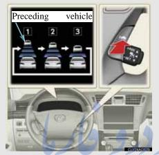
Pressing the button changes the vehicle-to-vehicle distance as follows:
