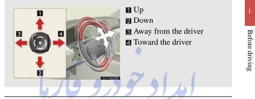
Automatic adjustment of the steering position
