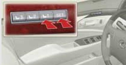
Press the "SET" button, then within 3 seconds press button "1", "2" or "3" until the signal beeps.
