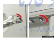
• The doors or trunk are unlocked using the mechanical key.
