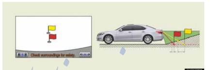
When the grade behind the vehicle slopes up sharply, objects appear to be farther away than they actually are.
