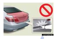
In the event that the trunk lid is left slightly open, the trunk easy closer will automatically close it to the fully closed position. It takes several seconds before the trunk easy closer begins to operate. Be careful not to catch fingers or anything else in the trunk lid, as this may cause bone fractures or other serious injuries
