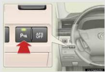
When on, the indicator light comes on and the buzzer sounds to inform the driver that the system is operational.
