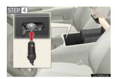
Connect the power plug to the power outlet socket.  $(\rightarrow P. 591)$
