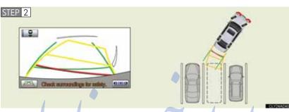
Turn the steering wheel so that the projected path guide lines are within the parking space, and back up carefully.
