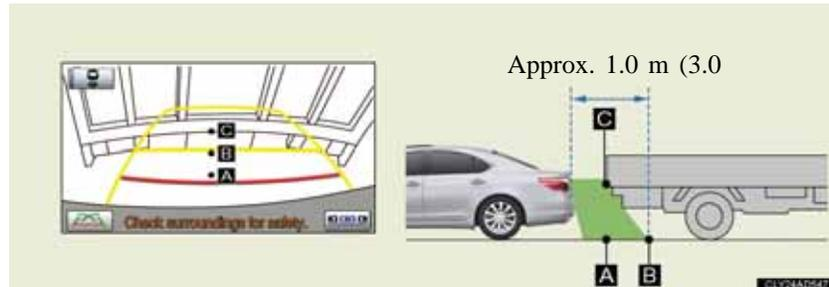
The distance that appears on the screen between three-dimensional objects (such as vehicles) and flat surfaces (such as the road) and the actual distance differ as follows.
