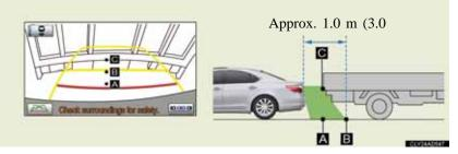
The distance that appears on the screen between three-dimensional objects (such as vehicles) and flat surfaces (such as the road) and the actual distance differ as follows.
