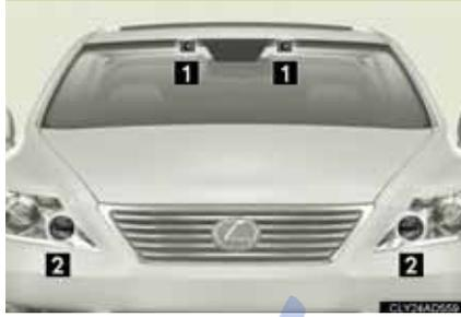
Detects pedestrians and other three-dimensional objects on or near the road ahead together with the radar sensor while the vehicle is moving. When the headlights are on, near-infrared rays are projected to ensure proper detection performance in the night time.
