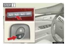
While pressing the desired button ("1", "2" or "3"), press and on the wireless remote control until the signal beeps.
