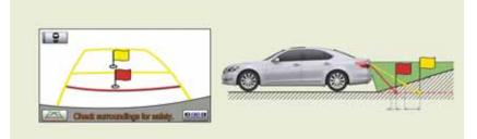
When the grade behind the vehicle slopes up sharply, objects appear to be farther away than they actually are.
