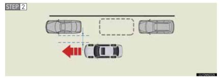
Move your vehicle slowly alongside the vehicle parked in front of the target parking space. Your vehicle should move parallel to the road or shoulder and be approximately 1 m (3 ft.) away from the side of the parked vehicle.
