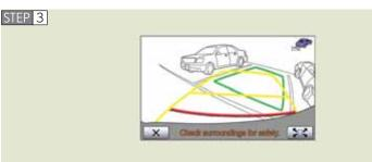
Position yourself as you would when backing up normally, and rest your hands on the steering wheel without applying any pressure. Check your surroundings and behind the vehicle for safety, and slowly back up, using the brake pedal to control the vehicle's speed.
