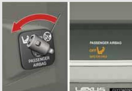
Insert the mechanical key into the cylinder and rotate to the off position. (→P. 35)
