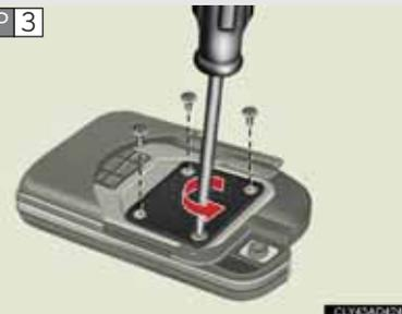
Remove the battery cover bolts and remove the battery cover.
