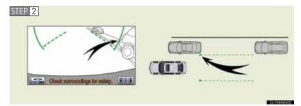
Back up until the point at which the green vertical line just overlaps the rear end of the parked vehicle. Then stop the vehicle.
