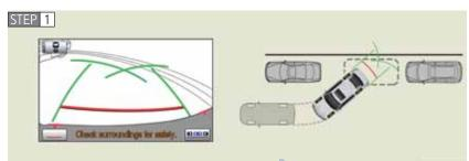
Place the shift lever in "R" position. Back up until the parking assist guide lines meet the edge of the desired parking location.
