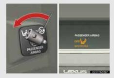
Insert the mechanical key into the cylinder and rotate to the off position.  $(\rightarrow P. 35)$
