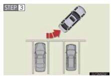
Position your vehicle so that you can enter the parking space, then stop the vehicle with the steering wheel straight.
