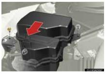
Remove the securing bolts and nut, and move the fuse block.
