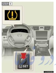
Push and hold the tire pressure warning reset switch until the tire pressure warning light blinks slowly 3 times and a message appears on the multiinformation display.
