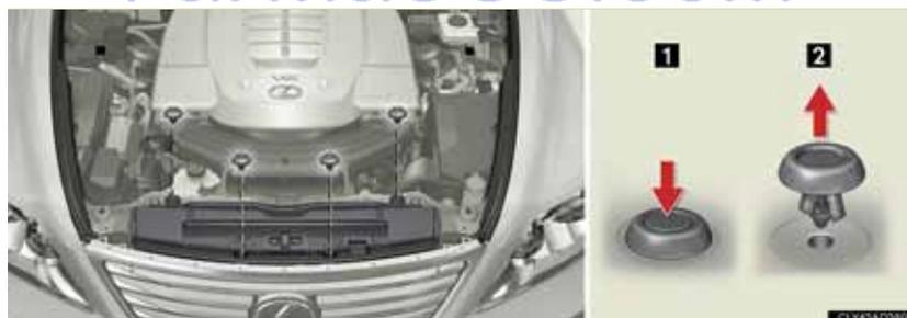
■ Installing the clips
