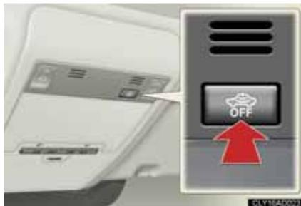
Turn the “ENGINE START STOP” switch OFF and press the intrusion sensor and tilt sensor cancel switch.
