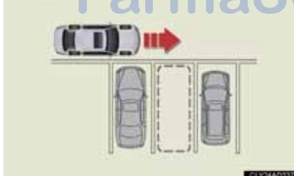
Move your vehicle slowly to a position perpendicular to and as close as possible to the target parking space.
