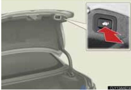
Pressing the switch closes the trunk lid automatically. (A buzzer sounds.)
