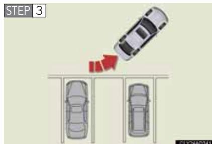
Position your vehicle so that you can enter the parking space, then stop the vehicle with the steering wheel straight.
