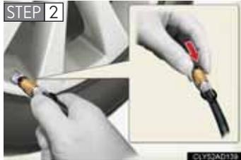
**STEP 2** Install the air release cap to the end of the hose and push the protrusion on the air release cap into the tire valve to let some air out.
