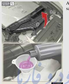
Add engine coolant if necessary.
