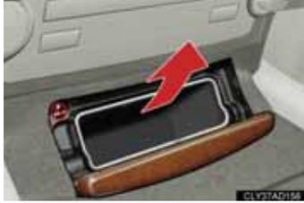
Holding the left edge of the non smokers box, pull upward.
