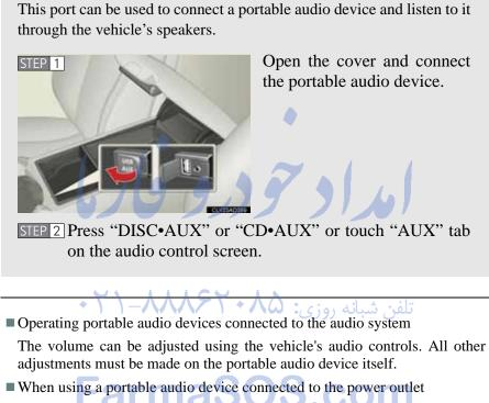
Noise may occur during playback. Use the power source of the portable audio device.
