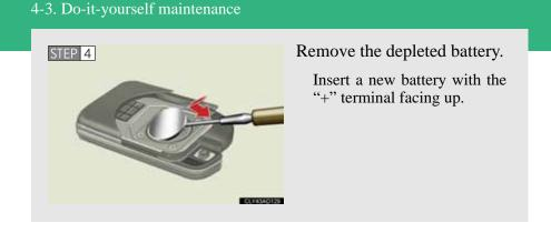
If the electronic key battery is discharged
