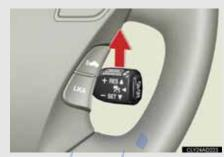
After the vehicle ahead of you starts off, push the lever up.
