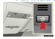
Turn the "ENGINE START STOP" switch OFF and press the intrusion sensor and tilt sensor cancel switch.
