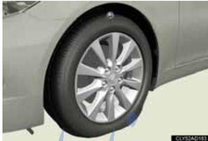
A tire should only be repaired with the emergency tire puncture repair kit if the damage is caused by a nail or screw passing through the tire tread.
