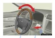
The green indicator light on the "ENGINE START STOP" switch will flash and a message will be shown on the multi-information display. Press the "ENGINE START STOP" switch again while turning the steering wheel left and right.
