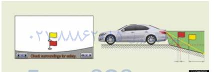
When the grade behind the vehicle slopes down sharply, objects appear to be closer than they actually are.
