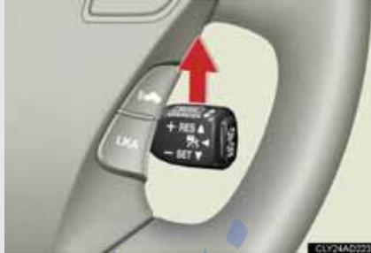
After the vehicle ahead of you starts off, push the lever up.
