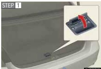
Lift up the handle and fold the trunk floor back.
