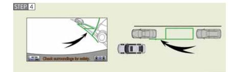
While the vehicle is stopped, turn the steering wheel. As you turn the steering wheel, the green outline will move to the location that your vehicle will move to and an extended green line will appear. Place the extended green line at the left of the rear tire of the parked vehicle.
