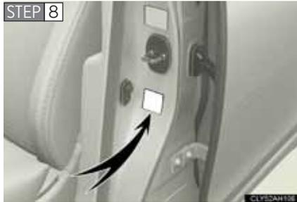
**STEP 8** Check the specified tire inflation pressure.
