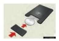
• If the battery was removed, reinstall the battery with the positive terminal facing the Lexus emblem.
