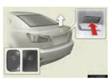
Press the button to unlock the trunk.
