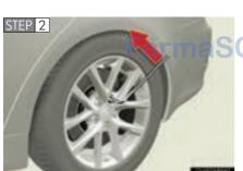
Slightly loosen the wheel nuts (one turn).
