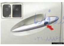
Press the lock button to lock the door.
