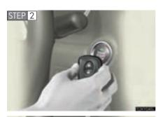
Touch the Lexus emblem side of electronic kev to the "ENGINE START STOP" switch.
