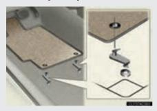
Fix the floor mat in place using the retaining hooks (clips) provided.
