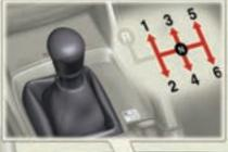
Fully depress the clutch pedal before operating the shift lever, and then release it slowly.
