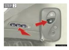
While the desired button ("1", "2" or "3") press on the wireless remote control until the signal beeps.
