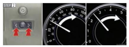
Push "<" or ">" within 6 seconds of the speedometer or tachometer needle moving to change the setting of the desired speed, then turn the indicator mode to "ON" by pushing the "ON/OFF" button.
