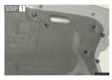
Open the trunk door and remove the trunk panel cover clips.
