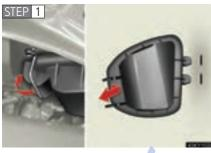
Release the lock and remove the cover.
