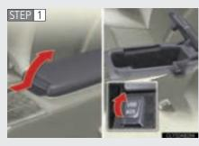
Open the cover and connect the portable audio device.
