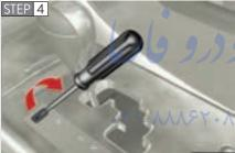
Pry the cover up with a flathead screwdriver or equivalent.
