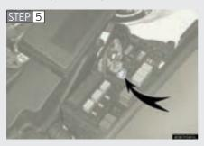
Remove the fuse with the pullout tool.
