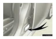
For the GAWR, see the Certification Label. For the maximum load of the tire, see the load limit at maximum cold tire inflation pressure mentioned on the sidewall of the tire.  $(\rightarrow P. 541)$ .
