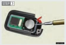
Remove the depleted battery.
