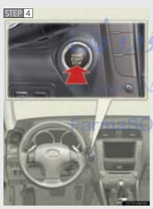
Press the "ENGINE START STOP" switch.
