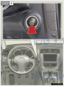
Press the "ENGINE START STOP" switch.
