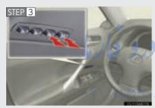
Push the "SET" button, then within 3 seconds push button "1", "2" or "3" until the signal beeps.
