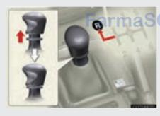
Shift the shift lever into the R position while lifting up the ring section.
