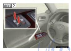
Shift the shift lever to P or N, press and hold the driver's door lock switch ( or or ) for about 5 seconds then release.
