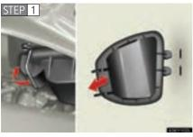
Release the lock and remove the cover.
