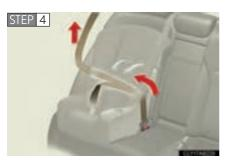
While pushing the child seat into the rear seat, allow the shoulder belt to retract until the child seat is securely in place.
