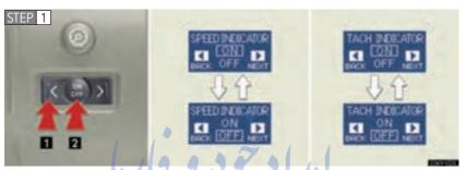
Push "<" or ">" to select the speed or tacho indicator set mode. (■) Turn the speed or tacho indicator to "OFF" and then "ON" by pushing the "ON/OFF" button. (■)
