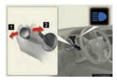
With the headlights on, push the lever forward to turn on the high beams.
