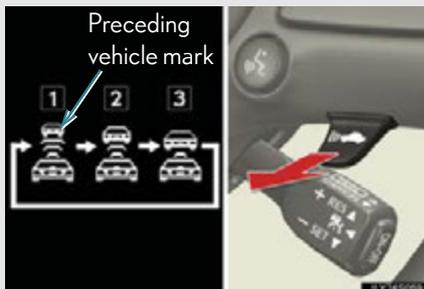
Each pull of the switch changes the vehicle-to-vehicle distance
