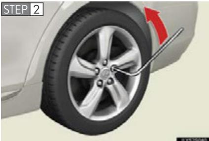
Slightly loosen the wheel nuts (one turn).
