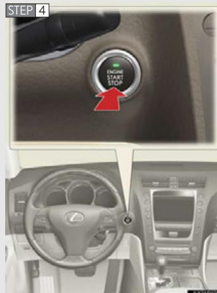
Press the "ENGINE START STOP" switch.
