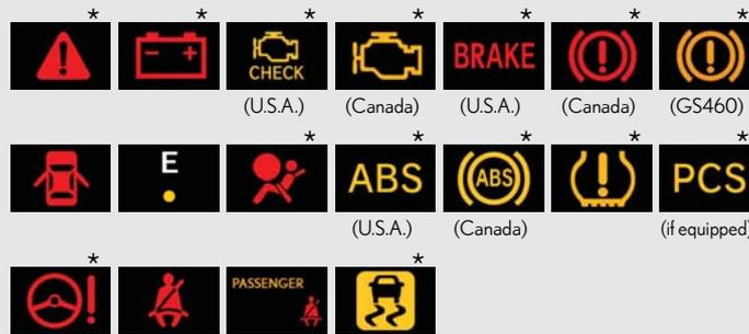
\*: These lights turn on when the "ENGINE START STOP" switch is turned to IGNITION ON mode to indicate that a system check is being performed. They will turn off after the engine is on, or after a few seconds. There may be a malfunction in a system if the lights do not come on, or turn off. Have the vehicle inspected by your Lexus dealer.
