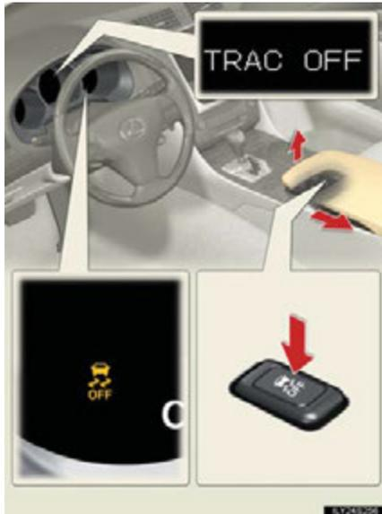
Push and hold the button for more than 3 seconds while the vehicle is stopped to turn off TRAC and Enhanced VSC.
