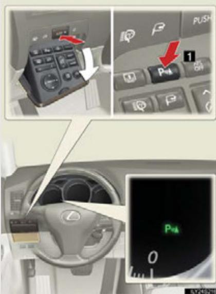
1 Press the switch to turn the system on/off.
