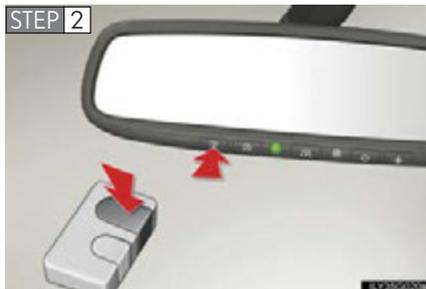
Press and hold one of the HomeLink<sup>®</sup> buttons and the transmitter button. When the HomeLink<sup>®</sup> indicator light changes from a slow to a rapid flash after 20 seconds, release both buttons.
