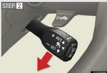
Accelerate or decelerate to the desired speed and press the lever down to set.
