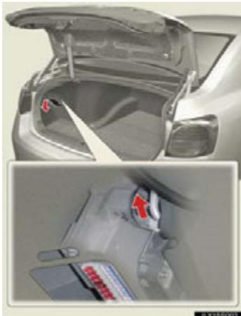
The lever can be used to open the fuel filler door if the fuel filler door cannot be opened using the inside switch because the 12 volt battery is discharged or for any other reason.
