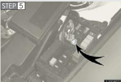
**STEP 5** Remove the fuse with the pull-out tool.
