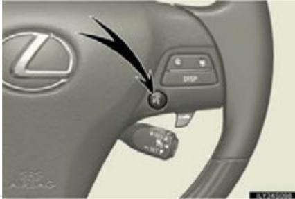
Press the talk switch to operate the voice command system. (→“Navigation System Owner’s Manual”)
