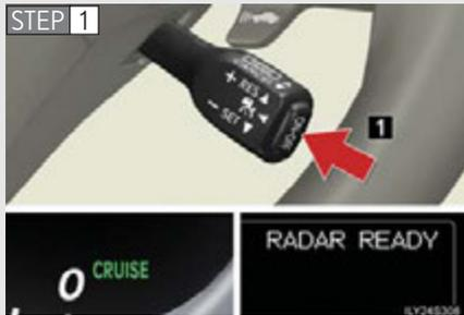
1 Press the “ON-OFF” button to activate the cruise control.
