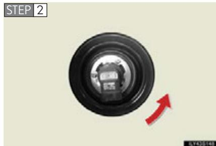
Turn the bulb base counterclockwise to remove it.
