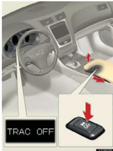
Quickly push and release the button to turn off TRAC.
