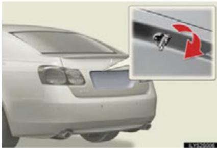
Turn the mechanical key clockwise to open.
