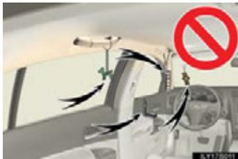
● Do not attach anything to areas such as the door, windshield glass, side door glass, front and rear pillars, roof side rail or assist grip.
