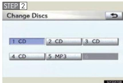
**STEP 2** Touch the desired disc on the screen or press  $\wedge$  or  $\vee$  on
