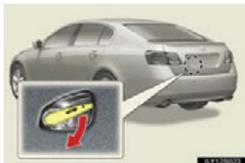
The trunk lid can be opened by pulling down on the glow-in-the-dark lever located on the inside of the trunk lid.
