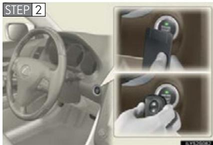
**STEP 2** Touch the Lexus emblem side of the electronic key to the “ENGINE START STOP” switch.
