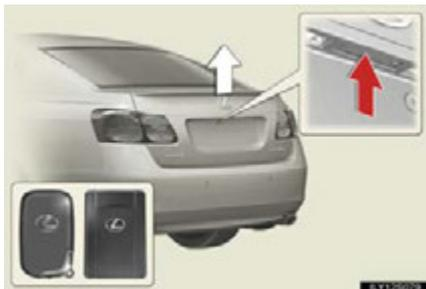
Press the button to unlock the trunk.
