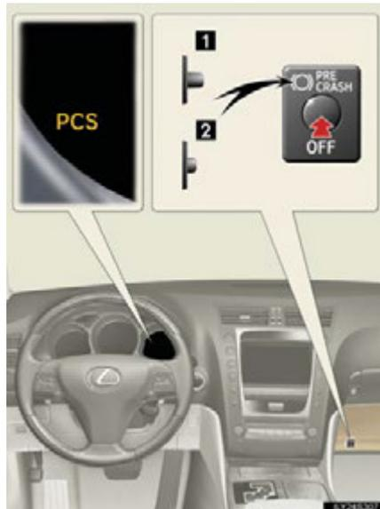
1 Pre-collision braking enabled
