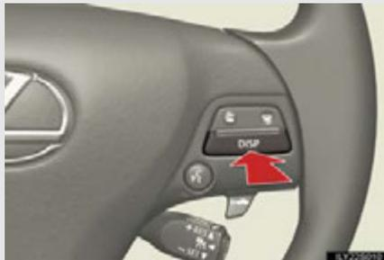
Display items can be switched by pushing the "DISP" switch.
