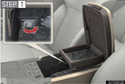
Connect the portable audio device.
