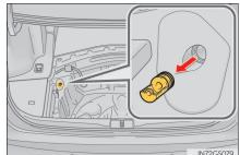
Insert the tool and press it down firmly while turning it counterclockwise until it stops.
