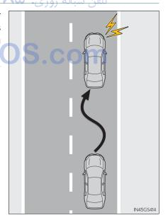
This function is linked with radar cruise control and provides the required assistance by operating the steering wheel to keep the vehicle in its current lane.
