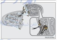
Align the tabs, and secure the mirror by pushing in each diagonally-opposite pair of tabs in order.
