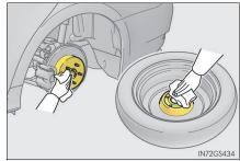
Install the tire and loosely tighten each wheel nut by hand by approximately the same amount.
