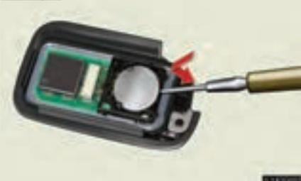
Remove the depleted battery.
