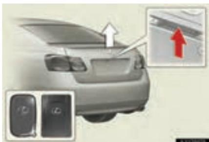
Press the button to unlock the trunk.
