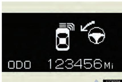
The steering guide symbol only shows the maneuvers necessary to avoid an obstacle.
