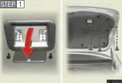
Open the trunk lid. Remove the trunk handle and panel cover clips.
