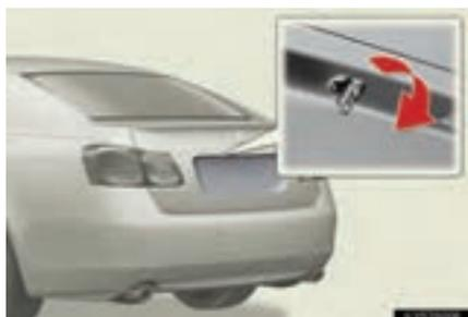
Turn the mechanical key clockwise to open.
