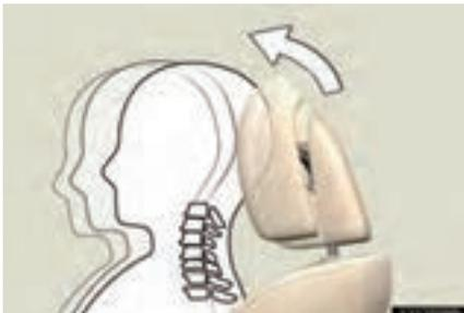
When the occupant's lower back presses against the seatback during a rear-end collision, the front portion of the head restraint moves slightly forward and upward to help reduce the risk of whiplash on the seat occupant.
