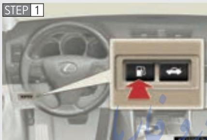
Press the fuel filler door opener switch.
