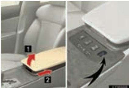
1 Pull up lever to release the lock.
