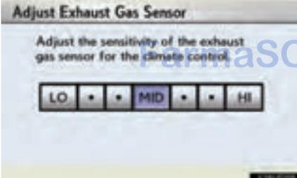
Touch any switch of "LO" to "HI" (lower sensitivity ↔ higher sensitivity) on the operating screen.
