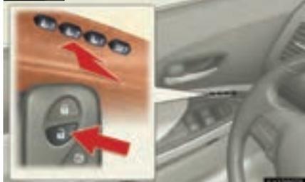
While pushing the desired button ("1", "2" or "3"), push
