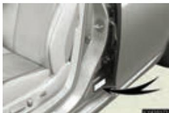
For the GAWR, see the Certification Label. For the maximum load of the tire, see the load limit at maximum cold tire inflation pressure mentioned on the sidewall of the tire. (→P. 602)
