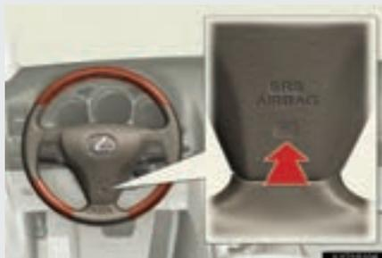
To sound the horn, press on or close to the
