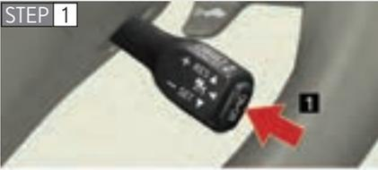
**1** Press the “ON-OFF” button to activate the cruise control.
