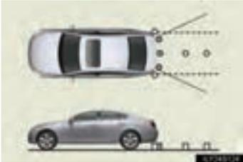
The area covered by the camera is limited. Objects which are close to either corner of the bumper or under the bumper cannot be seen on the screen.
