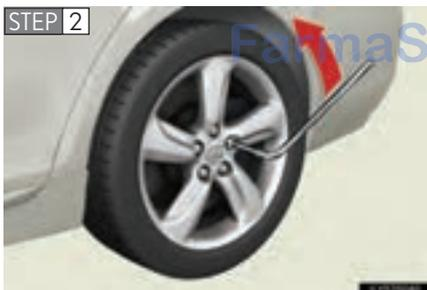
Slightly loosen the wheel nuts (one turn).
