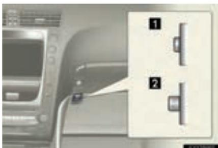
Turn the main switch in the glove box OFF to disable the trunk opener.
