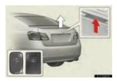
Press the button to unlock the trunk.
