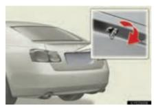
Turn the mechanical key clockwise to open.
