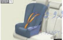
Place the child restraint system on the seat facing the front of the vehi-
