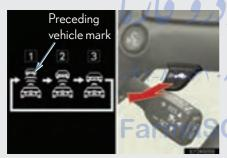
Each pull of the switch changes the vehicle-to-vehicle distance
