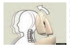
When the occupant's lower back presses against the seatback during a rear-end collision, the front portion of the head restraint moves slightly forward and upward to help reduce the risk of whiplash on the seat occupant.
