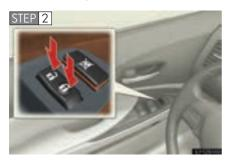
Shift the shift lever to "P" or "N", press and hold the driver's door lock switch ( a or approximately 5 seconds and then release.
