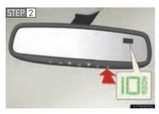
Press and hold the switch. A number (1 to 15) appears on the compass display.
