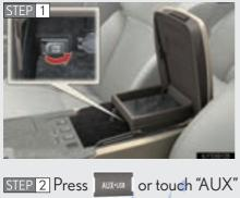
Connect the portable audio device.
