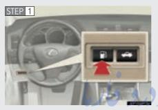
Press the fuel filler door opener switch.
