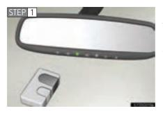
Point the remote control transmitter for the device 1 to 3 in. (25 to 75 mm) from the HomeLink<sup>®</sup> control buttons.
