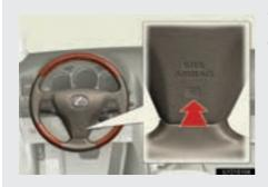
To sound the horn, press on or close to the born mark.
