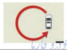
If "CAL" appears on the display, drive the vehicle at 5 mph (8 km/h) or less in a circle until a direction is displayed.
