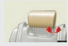
Grip head restraint and twist to tilt forward or backward.
