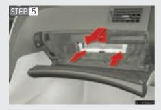
Press the tabs and remove the filter case.
