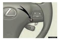
Press the talk switch to operate the voice command system. (→"Navigation System Owner's
