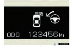
The steering guide symbol only shows the maneuvers necessary to avoid an obstacle.
