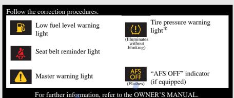
\*: It also comes on due to natural causes such as natural air leaks and tire inflation pressure changes caused by temperature. Adjust the tire inflation pressure to the
