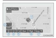
To scroll over the map screen, place the cursor mark in the desired position and then press and hold the Remote Touch knob.
