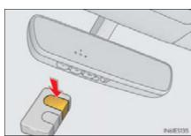
Press and hold the handheld transmitter button until the HomeLink<sup>®</sup> indicator light changes from slowly flashing orange to rapidly flashing green (rolling code) or continuously lit green (fixed code), then release the button.
