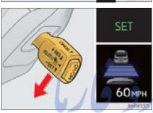
1 Press the "ON/OFF" button to activate the cruise control.
