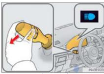
Push the lever away from you with the headlight switch in the AUTO or position.
