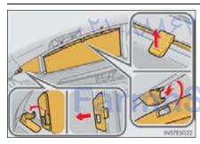
Pull the tab of the rear door sunshade and hook the sunshade on the anchors.
