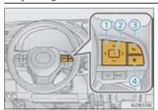
The multi-information display is operated using the meter control switches.
