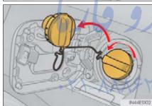
Turn the fuel tank cap slowly to open and hang it on the back of the fuel filler door.
