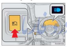
Press the Automatic High Beam switch.
