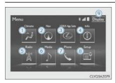
Press the "MENU" button on the Remote Touch to display the "Menu" screen.
