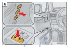
While pressing the recalled button, press and hold the door lock switch (either lock or unlock) until the buzzer sounds.
