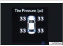
The tire pressure detected by the tire pressure warning system can be displayed on the multi-information display. ( $\rightarrow$ P.28)
