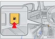
1 Press the opener switch to open the fuel filler door.
