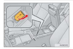
Open the console box, open the cover and connect the portable audio device.
