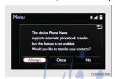
**2** To transfer new contacts from a cellular phone, select "Always" and then enable "Automatic Transfer". Select "Once" if you want to transfer new contacts from a cellular phone.
