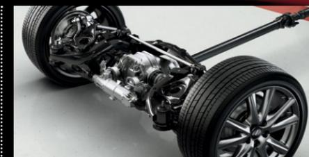
the front for optimal agility and control. At low speeds, the rear wheels turn in the opposite direction for precise maneuvering and a tighter turning circle. All the while, the Variable Gear-Ratio Steering (VGRS) system provides optimized responsiveness and a more direct steering feel.
