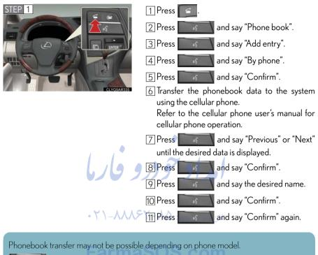
Pressing this switch turns the speech command system on. Say a command after the beep.
