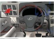
► Instrument panel To open or close the back door, press the switch.
