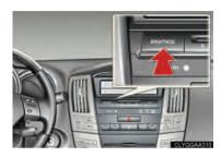
To adjust the brightness of the multi-display light, press the button repeatedly until the desired brightness is obtained.
