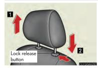
To raise: push the head restraint upward.
