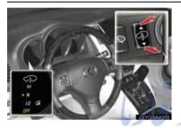
To select a height mode, press  $\blacktriangle$  or  $\blacktriangledown$  on the height select switch.
