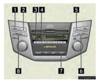
All tracks in current disc: press First track of each CD: press and hold Eject Random playback Current disc: press All discs: press and hold Repeat Current track: press Current disc: press and hold Disc load Disc select Text information Track select/rewind/fast-forward
