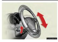
To adjust the steering wheel, pull the lever up while holding the steering wheel, tilt the steering wheel to the desired angle, and release the lever.
