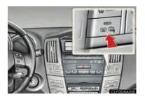
To defog the rear window and the outside rear view mirrors, press the button.
