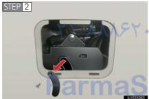
Remove the screw and cover. (Vehicle without power back door)
