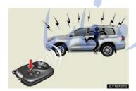
When (i) is pressed for longer than about one second, the head lights/tail lights/emergency flashers will flash, the front and rear interior lights will come on, and an alarm will sound for about 60 seconds to deter any person from trying to break into or damage your vehicle.
