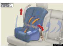
While pushing the child restraint system into the second seat, allow the shoulder belt to retract until the child restraint system is securely in place.
