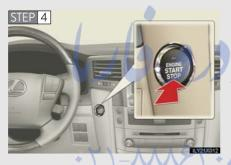
Press the "ENGINE START STOP" switch.
