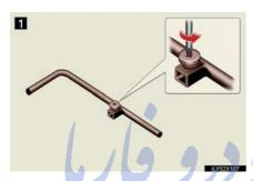
**1** Loosen the screw using a screwdriver.
