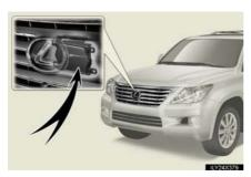
When traveling on a road with very light traffic and very little to reflect the radar waves emitted by the radar sensor, the system may decide that the radar sensor is dirty, even if the sensor is not actually dirty. The system will automatically restore itself when reflected radar waves are detected.
