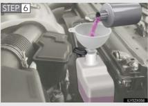
Add engine coolant if necessary.
