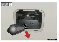
Push the lever with the back door motor, open the back door.
