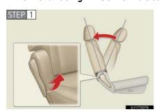
Fold the seatback while pulling the seatback angle lever. Return the seatback and secure it at the first lock position. (→P. 66)
