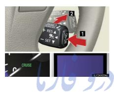
■ Press the "ON-OFF" button to activate the cruise control.
