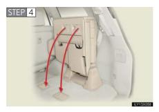
Remove the seat hook covers from the underside of the seat cushion, and install them on the seat hooks.
