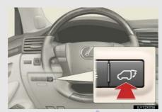
The power back door can be opened/closed using the power back door switch or wireless remote control.  $(\rightarrow P. 45)$
