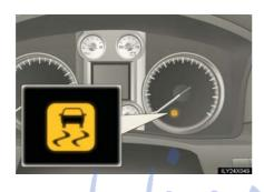
If the vehicle is in danger of slipping, rolling backwards when starting on an incline, or if the wheels spin, the slip indicator light flashes to indicate that the VSC/Active TRAC/hill-start assist control systems have been engaged.
