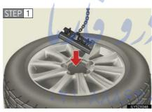
Lay down the tire with the outer side facing up, and install the holding bracket.
