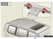
Turn the knobs counterclockwise to release the cross rails.
