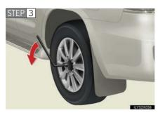
Slightly loosen the wheel nuts (one turn).
