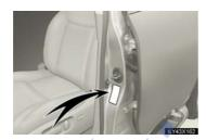
For the GAWR, see the Certification Label. For the maximum load of the tire, see the load limit at maximum cold tire inflation pressure mentioned on the sidewall of the tire.  $(\rightarrow P. 697)$
