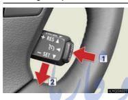
Press the "ON-OFF" button. The system will turn on.
