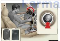
The steering lock is engaged when the driver's door is opened with the "ENGINE START STOP" switch OFF.
