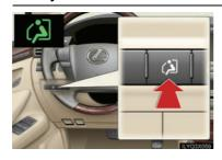
To select a height mode, shift the height select switch forward or backward.
