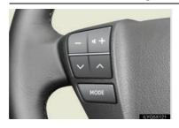
**"MODE"**: Turns the audio system on/off, or changes the audio mode.
