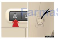
Designed for use with electrical appliances. To use the power outlet, push the "AC 115V" switch on the instrument panel.
