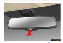
To turn automatic mode on/off, press the "AUTO" button. The indicator comes on when automatic mode is turned on.
