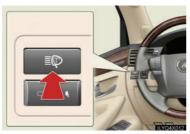
The headlight cleaner can be used only when the "ENGINE START STOP" switch is in IGNITION ON mode and the headlights are on.
