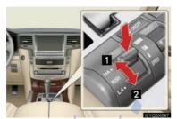
► Center differential lock/unlock switch
