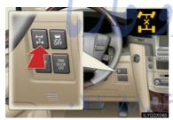
To select "L4" mode, push down and shift the switch backward. To select "H4" mode, shift the switch forward.
