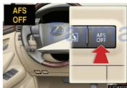
The system can be turned on and off using the "AFS OFF" switch.
