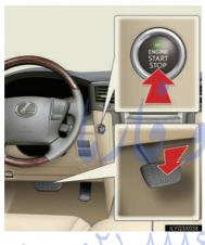
Make sure the parking brake is engaged and the shift lever is in "P".
