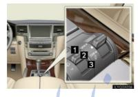
To select a driving mode, shift the damping mode select switch forward or backward.
