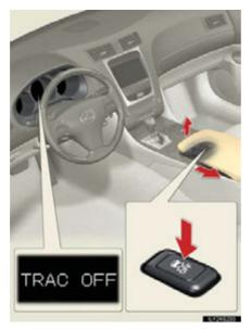
Quickly push and release the button to turn off TRAC.
