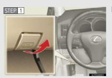
Release the lock from the inside of the vehicle to open the hood.
