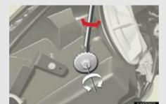
Using a Phillips-head screwdriver, turn adjustment bolt A so that the bubble is within the 2 center lines.
