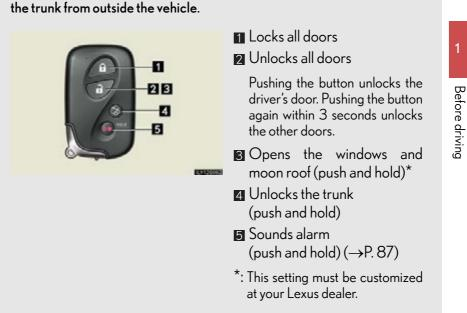
The wireless remote control can be used to lock and unlock the vehicle and
