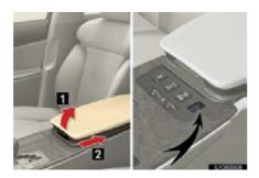
Pull up lever to release the lock.
