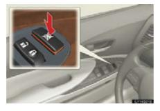
Press the switch down to lock passenger window switches.
