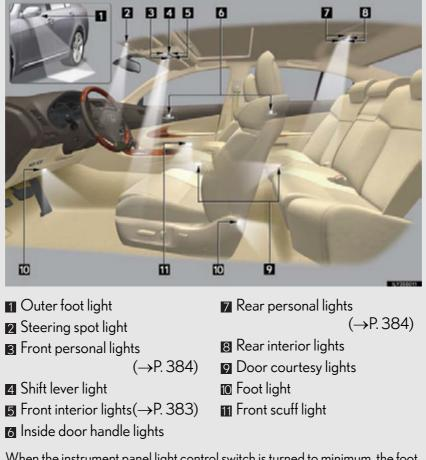
When the instrument panel light control switch is turned to minimum, the foot lights, inside door handle lights and shift lever light will turn off.  $(\rightarrow P. 146)$
