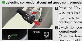
Press the "ON-OFF" button to activate the cruise control.
