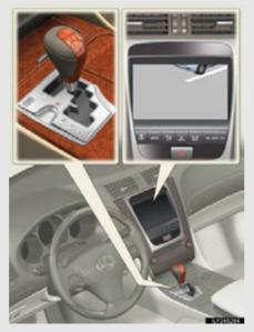
Rear view image is displayed when the shift lever is in "R".
