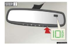
Press and hold the switch. A number (1 to 15) appears on the compass display.
