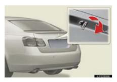
Turn the mechanical key clockwise to open.
