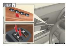
While pushing the desired button ("1", "2" or "3"), push the lock or unlock side on the door lock switch (either the driver or passenger side) until the signal beeps.
