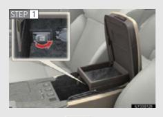
Connect the portable audio device.
