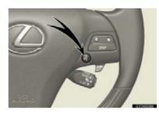
Press the talk switch to operate the voice command system. (→"Navigation System Owner's Manual")
