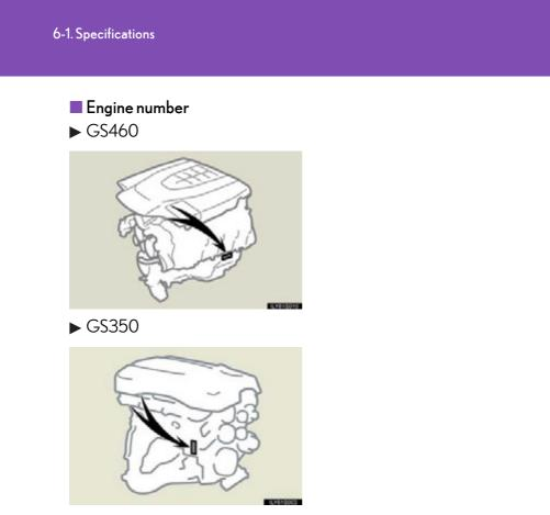
The engine number is stamped on the location as shown.
