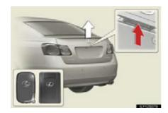
Press the button to unlock the trunk.
