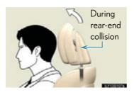
Even small forces applied to the seatback may cause the head restraint to move.
