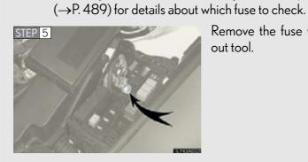
Remove the fuse with the pullout tool.
