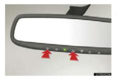
Press and hold the 2 outside buttons for 20 seconds until the indicator light flashes.
