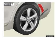
Slightly loosen the wheel nuts (one turn).
