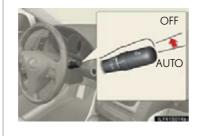
Set the wiper switch to off. If the wiper switch is in "AUTO", the wipers may operate and the wiper blades may be damaged.
