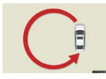
If "CAL" appears on the display, drive the vehicle at 5 mph (8 km/h) or less in a circle until a direction is displayed.
