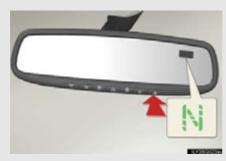
To turn the compass on or off, press the button for more than 3 seconds.
