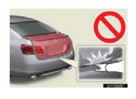
In the event that the trunk lid is left slightly open, the trunk easy closer will automatically close it to the fully closed position. It takes several seconds before the trunk easy closer begins to operate. Be careful not to catch fingers or anything else in the trunk lid, as this may cause bone fractures or other serious injuries.
