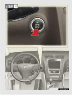
Press the "ENGINE START STOP" switch.
