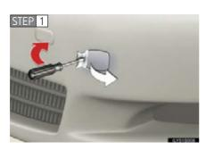
Remove the eyelet cover using a flathead screwdriver.
