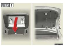
Open the trunk lid. Remove the trunk handle and panel cover clips.
