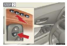
While pushing the desired button ("1", "2" or "3"), push and on the wireless remote control until the signal beeps.
