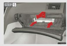
Press the tabs and remove the filter case.
