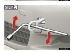
Tighten down the towing eyelet securely using a wheel nut wrench.
