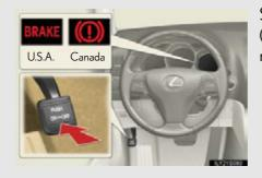
Sets the parking brake<sup>\*</sup> (Depressing the pedal again releases the parking brake.)
