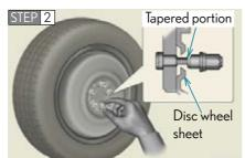
Remove any dirt or foreign matter from the wheel contact surface.
