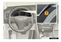
If the vehicle is in danger of slipping, rolling backwards when starting on an incline, or if the rear wheels (2WD models) or all wheels (4WD models) spin, the slip indicator light flashes to indicate that the Enhanced VSC/ TRAC/hill-start assist control systems have been engaged.
