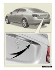
The area covered by the camera is limited. Objects which are close to either corner of the bumper or under the bumper cannot be seen on the screen.
