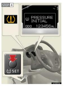
Push and hold the tire pressure warning reset switch until the tire pressure warning light blinks slowly three times and the mes-"PRESSURE INITIAL" sage appears on the multi-information display.
