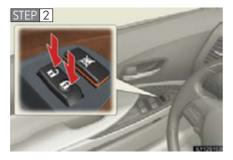
Shift the shift lever to "P" or "N", press and hold the driver's door lock switch ( or ) for approximately 5 seconds and then release.
