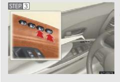
While pushing the "SET" button, or within 3 seconds after the "SET" button is pushed, push button "1", "2" or "3" until the signal beeps.
