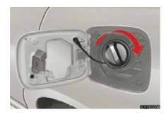
After refueling, turn the fuel tank cap clockwise until you hear a click. The cap will revolve slightly in the opposite direction once released.
