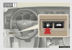
Press the fuel filler door opener switch.
