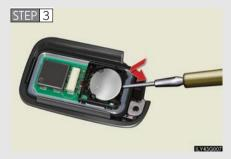
Remove the depleted battery.
