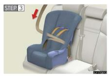
Fully extend the shoulder strap and then allow it to retract slightly into the ALR lock mode.
