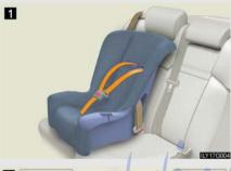
■ Seat belts equipped with a child restraint locking mechanism (ALR/ELR belts except driver's seat belt)
