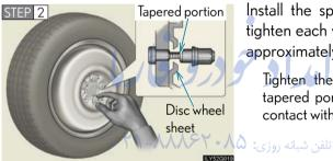
Install the spare tire and loosely tighten each wheel nut by hand to approximately the same amount.
