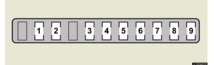
Fuse Ampere Circuit RR S/SHADE 7.5 Rear sunshade 1 30 Pre-collision seat belt 2 **PSB** 10 RR-IG2 3 Pre-collision seat belt, seat belt pre-10 RR-IG1 4 tensioners, A/P UNIT, rear sunshade 10 RR-B Trunk light, noise filter 5 **RR FOG** 7.5 6 10 STOPLPL Stoplights, back-up light 7 STOP LP R 10 High mounted stoplights 8 Tail lights, license plate lights, rear **RR TAIL** 10 9 side marker lights
