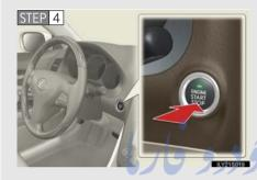
Press the "ENGINE START STOP" switch.
