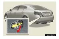
The trunk lid can be opened by pulling down on the glow-in-the-dark lever located on the inside of trunk lid.
