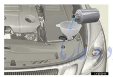
If any washer does not work or the warning message appears on the multi-information display. washer tank may be empty. Add washer fluid.
