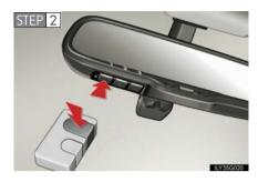
Press and hold one of the buttons on the HomeLink<sup>®</sup> and the button on the transmitter. When the indicator light on the HomeLink<sup>®</sup> changes from a slow to a rapid flash after 20 seconds, you can release both buttons.
