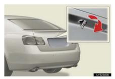
Turn the mechanical key clockwise to open.
