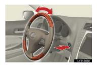
The green indicator light on the "ENGINE START STOP" switch will flash and a message will be shown on the multi-information display. Press the "ENGINE START STOP" switch again while turning the steering wheel left and right.
