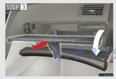
Open the glove box and remove the partition.
