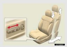
Head restraint height can be adjusted automatically along with the seat position adjustment.  $(\rightarrow P. 45)$
