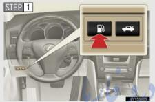
Press the fuel filler door opener switch.
