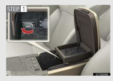
Connect the portable audio device.
