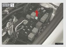
Remove the fuse with the pullout tool.
