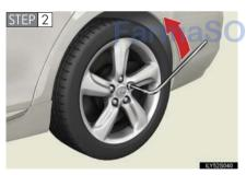
Slightly loosen the wheel nuts (one turn).
