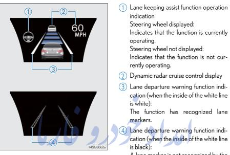
A lane marker is not recognized by the system, or the LKA system functions are temporarily canceled.
