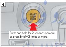
To stop the engine, press and hold the engine switch for 2 consecutive seconds or more, or press it briefly 3 times or more in succession.
