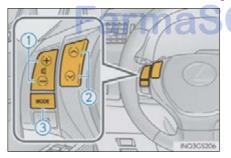
Radio mode: Selects a radio station SAT mode: Selects a channel Audio CD mode: Selects a track MP3/WMA/AAC disc mode: Selects a file DVD mode: Selects a chapter USB mode: Selects a file/track iPod mode: Selects a track/file BT audio mode: Selects a track
