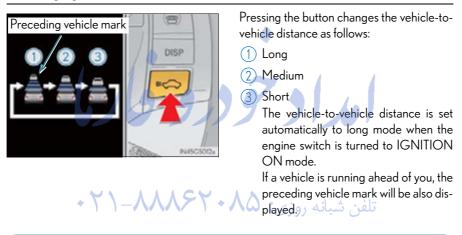
The vehicle-to-vehicle distance control mode maintains the preset cruising speed as long as no vehicle is detected ahead.
