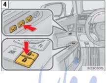
While pressing the recalled button, press and hold the door lock switch (either lock or unlock) until the buzzer sounds.
