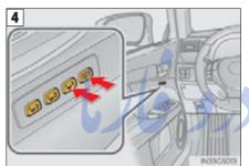
While pressing the "SET" button, or within 3 seconds after the "SET" button is pressed, press button "1", "2" or "3" until the buzzer sounds.
