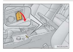
Open the console box, open the cover and connect the portable audio device.
