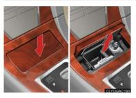
To remove the ashtray, push the back part of the lid and pull the ashtray upwards.
