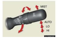
MIST: operates once AUTO: automatic operation\* LO: low speed HI: high speed \*: Sensitivity can be adjusted by turning the band.
