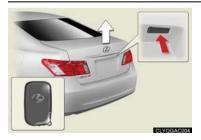
To open the trunk, press and hold the trunk release button.
