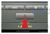
Engaging the emergency flasher switch causes all the turn signal lights to flash.
