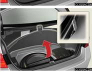
The lever can be hooked on the edge of the trunk.
