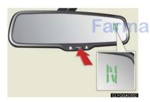
To display the compass, press and hold the AUTO button for 3 or more seconds.
