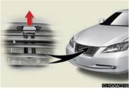
[2] Insert your fingers under the hood, pull the hood catch up and lift the hood.
