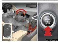
The steering wheel locks when the "ENGINE START STOP" switch is in OFF mode.
