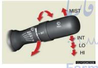
MIST: operates once INT: intermittent operation\* LO: low speed HI: high speed \*: Wiper interval can be adjusted by turning the band. تلفن شبانه روزی: To spray washer fluid, pull the lever.
