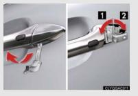
To unlock or lock the vehicle, use the mechanical key to remove the lock cover on the driver's door handle. The mechanical key is stored inside the electronic key.
