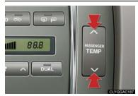
In DUAL mode, driver and passenger side temperature settings can be adjusted separately.
