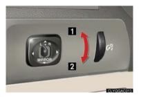
**1** To brighten: turn the knob upward. **2** To dim: turn the knob downward.
