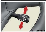
To increase speed: push the lever up. To decrease speed: push the lever down.
