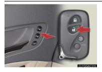
While holding down the desired memory button, press and hold a on the wireless remote control until you hear a beep.
