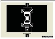
Sensors are used to detect obstacles near the vehicle. The distance to a detected obstacle is shown by the number of indicator bars.
