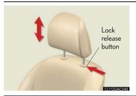
To raise: pull the head restraint upward. To lower: push the head restraint down while pressing the lock release button.
